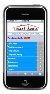
Scrolling down the list of the Function pages, you will find the setup access for the rooms: if only the checkbox "View" is selected, the user will only be able to see lights, temperatures, alarm status,..., but not to control them. In this case the symbol  $\bigotimes$  will be shown on the red side of the function.
